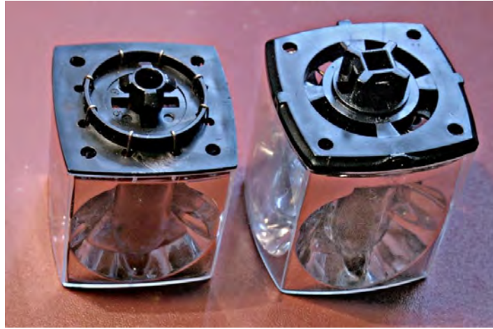
Figure 3. Flashcube (Left) and Magicube (Right) for Kodak® Instamatic Cameras Circa 1970-1980s (Kodak, 2011)
