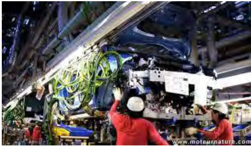
Figure 10. Nissan Leaf Production Line (2011)
